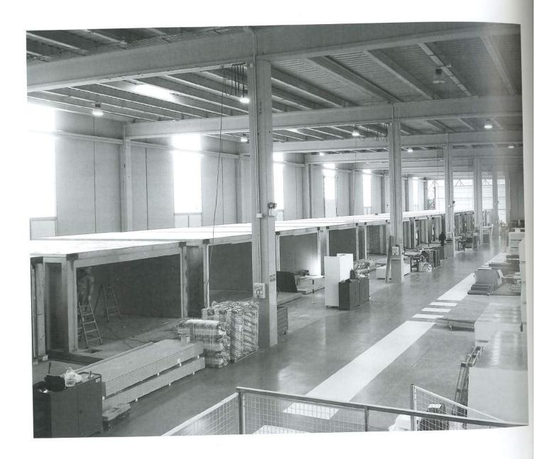
5.3.22 Off-site facility accommodating assembly line, fabrication, and installation equipment Source: © Compact Hablt, 2014.
